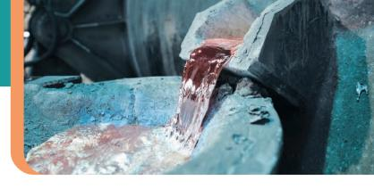
in contact with melted metal, preventing aluminum from adhering to those structures.
